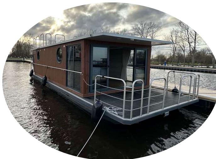
Aluminum frame, isolated windows system. Bow sliding doors; not-opening starboard and port vitrine windows; sliding bedroom vitrine window on the port side; not-opening wooden frame, round windows in the port and starboard side; the glass: single-chamber, double-layer, tempered, tinted.
